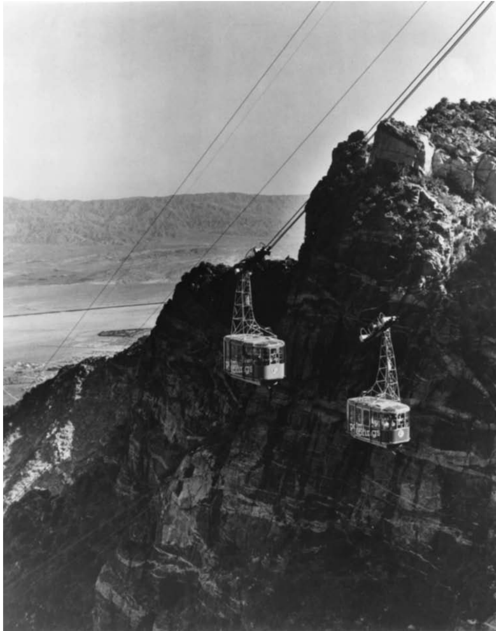
Trams and cable cars can greatly enhance visitors' abilities to enjoy many different views of a destination. Here, the halfway point on the Palm Springs tram's journey from the 2643-foot Valley Station to the 8516-foot Mountain Station is reached when the two cars pass between towers two and three. At this point, the two cars are thirty-four feet apart. Photo courtesy of the Palm Springs Aerial Tramway.
