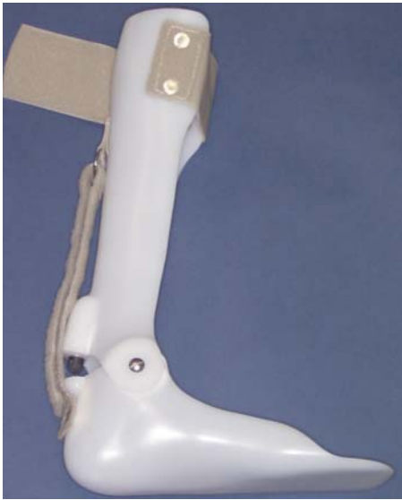
Figure 5.17. There are a group of children who are smaller, especially with some plano-valgus foot deformity, in whom some ankle motion is thought to be beneficial. One alternative is to use a standard articulated AFO and attach a posterior restraining strap to prevent hyperdorsiflexion. Although this seems like a good goal, unless the child is very light, there does not seem to be any cloth material that can be attached to the orthotic that does not rapidly stretch out.
