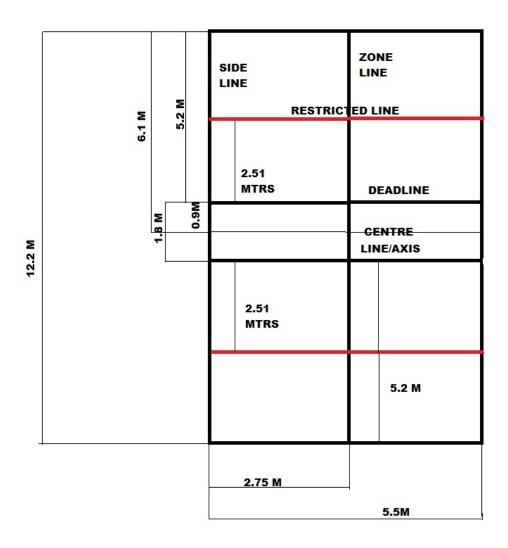
(all dark lines are to be 5cm thick) (the thin lines are the dimension lines)
